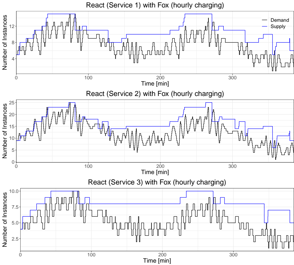
Figure 11.9: Scaling behavior of React with Fox on the BibSonomy trace with hourly charging scheme.
