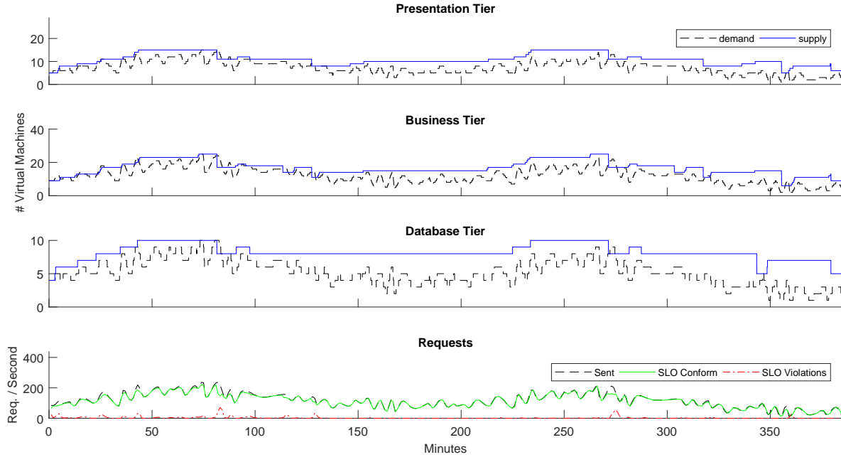
Figure 6: Scaling behavior of React with FOX on the BibSonomy trace with Amazon EC2 cost model.
