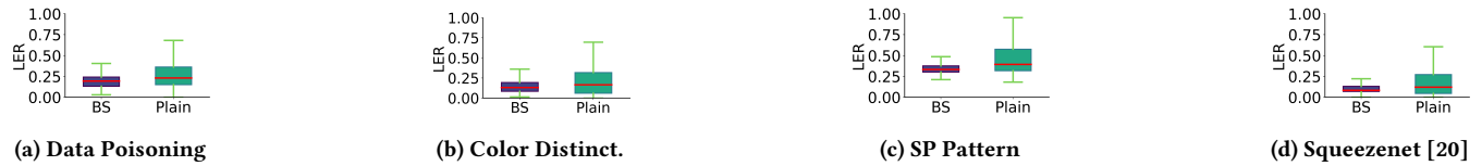
Figure 6: Levenshtein error rates (LER) without (Plain) and with beam search error correction (BS) for varying scenarios.
