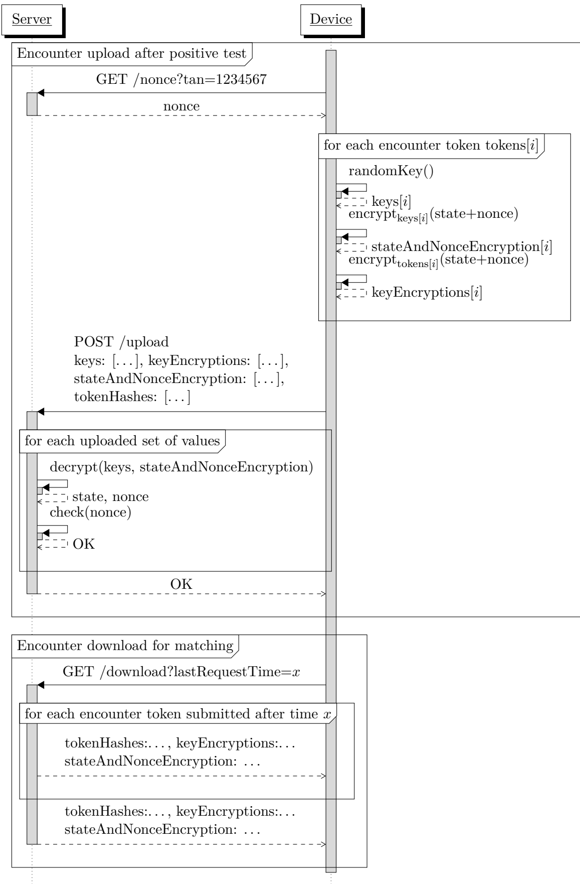
Figure 2.5.: Sequence diagram of server-device communication in TraceCORONA
