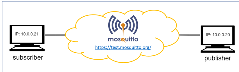
Fig. 8. The setup used to gather data of the network quality between the MQTT clients and the public MQTT Mosquitto broker.
